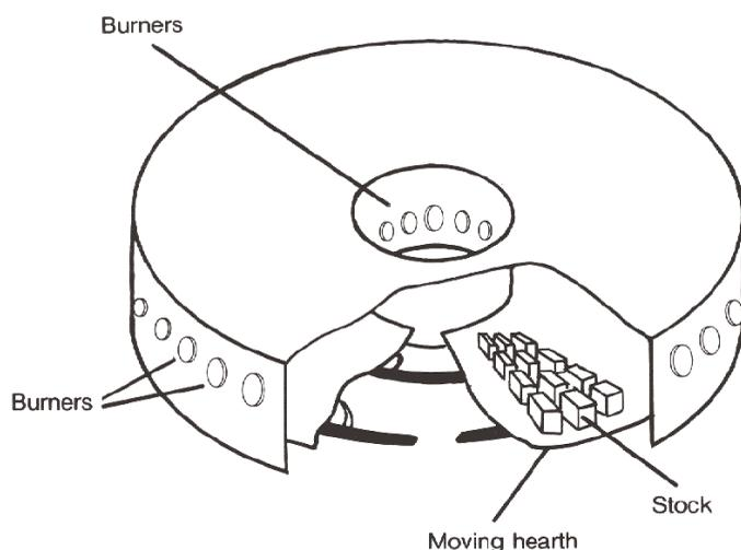
**Figure 4.6 Rotary Hearth Type Furnace**
