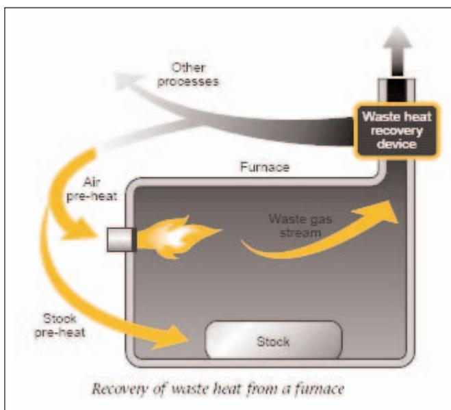
Figure 4.20 Waste Heat Recovery from a Furnace
