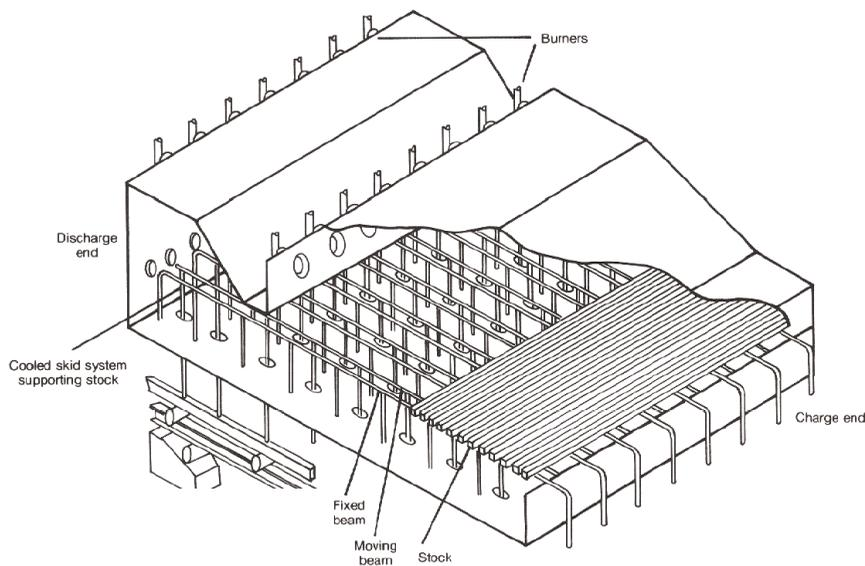
Figure 4.8 Walking Beam Type Furnace
