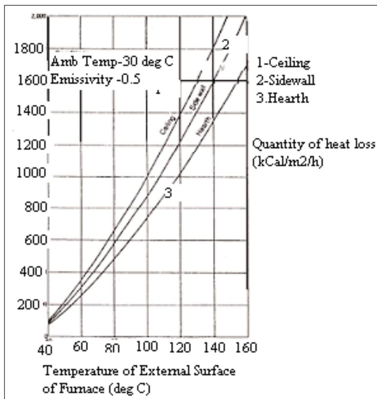
Figure 4.26 Quantity of Heat Release at Various Temperatures
