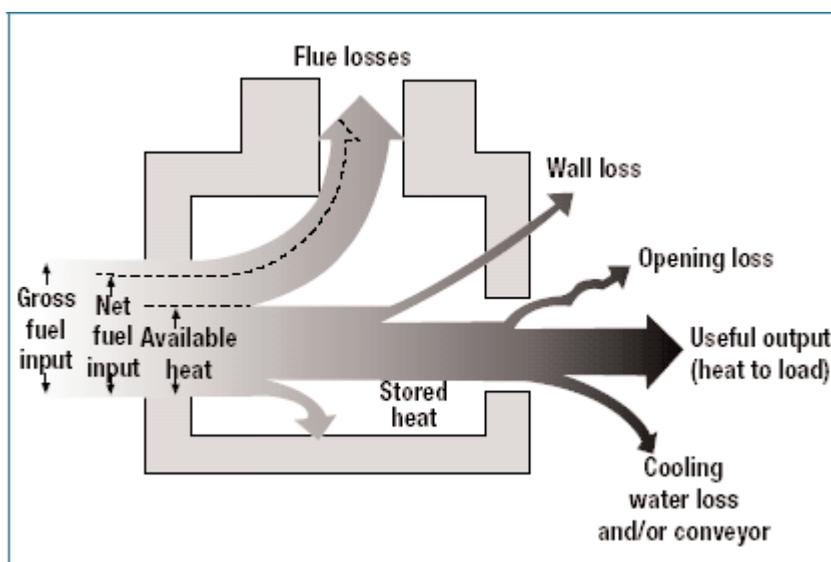
Figure 4.9 Heat Losses in Industrial Heating Furnaces
