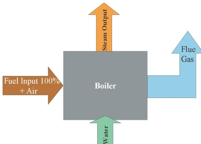
$$\text{Efficiency} = \frac{\text{Heat addition to Steam} \times 100}{\text{Gross Heat in Fuel}}$$
