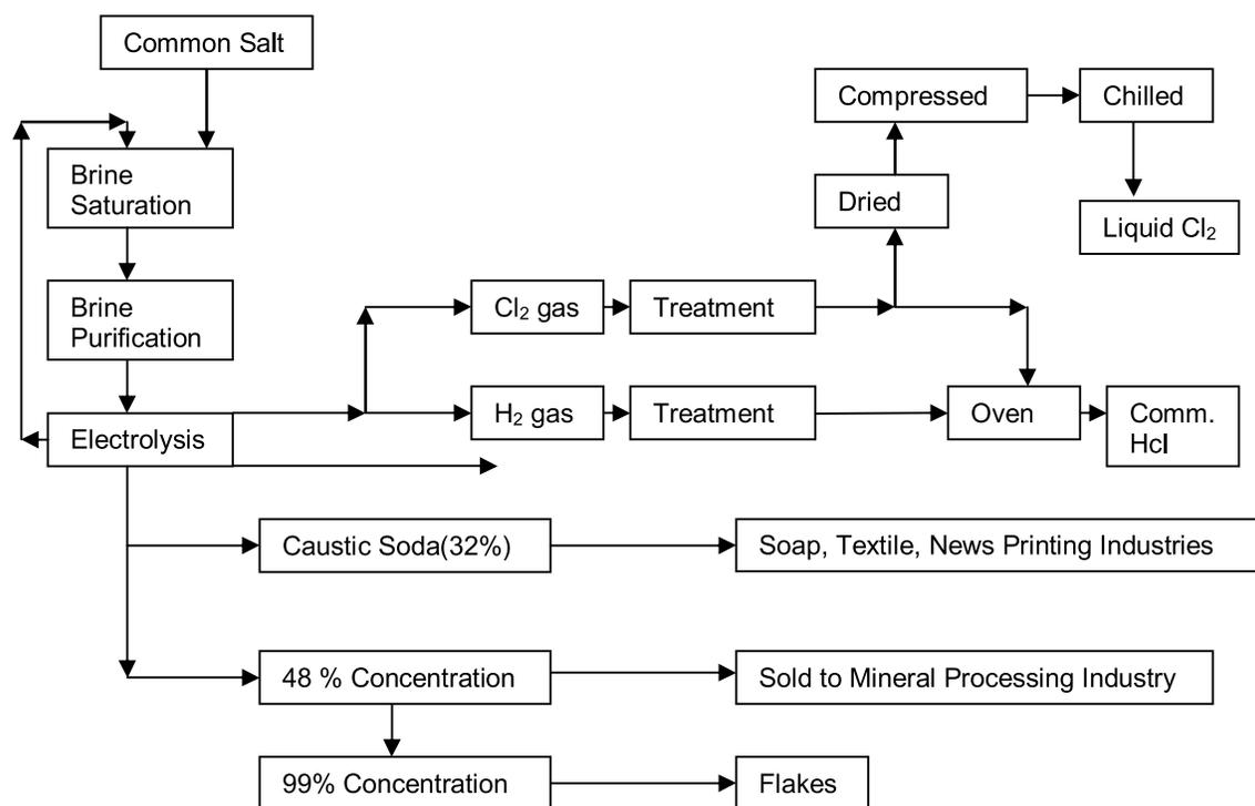
Process Flow Chart for Caustic Soda, Liq. Cl<sub>2</sub> & HCl Production in Caustic soda plant.
