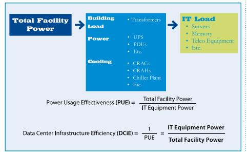
NOTE: Improving PUE from 2.0 to 1.6 for a Data Center with a 2.5 MW IT load yields a 20% energy savings or over INR 50 lakhs annual savings at INR 5 /kWh.
