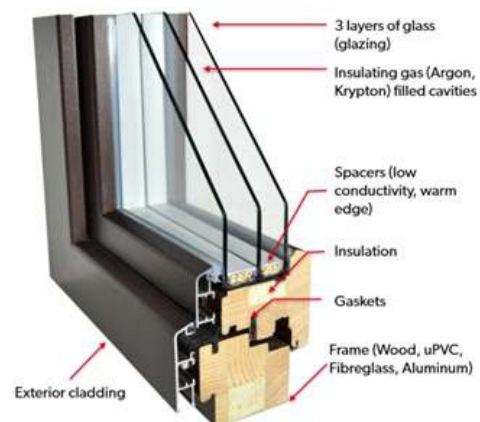
FIGURE 16 HIGH PERFORMANCE GLAZING SYSTEM
