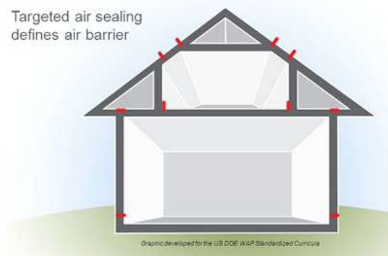
FIGURE 11 ENVELOPE AIR TIGHTNESS
