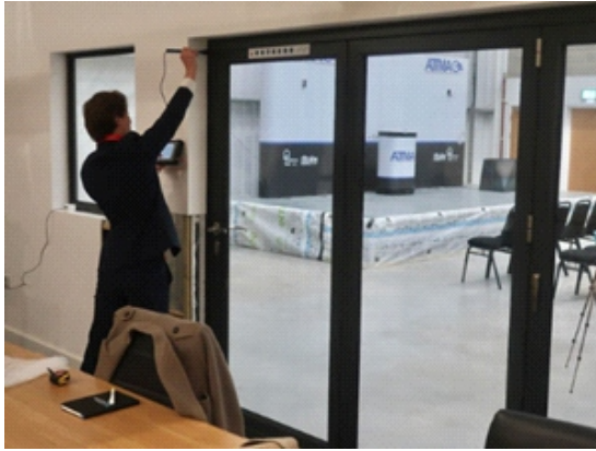
FIGURE 5 WINDOW- AIR TIGHTNESS
