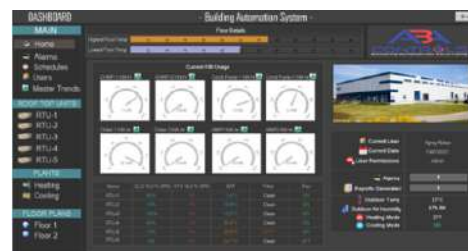
FIGURE 40 ADVANCED BUILDING MANAGEMENT SYSTEM
