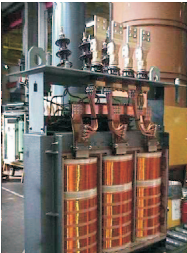
Figure 10.9 1600 kVA Amorphous Core Transformer
