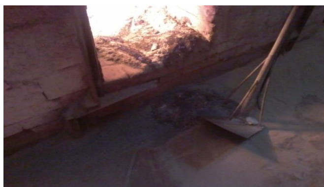
Figure 12: Ash removal opening in roaster
