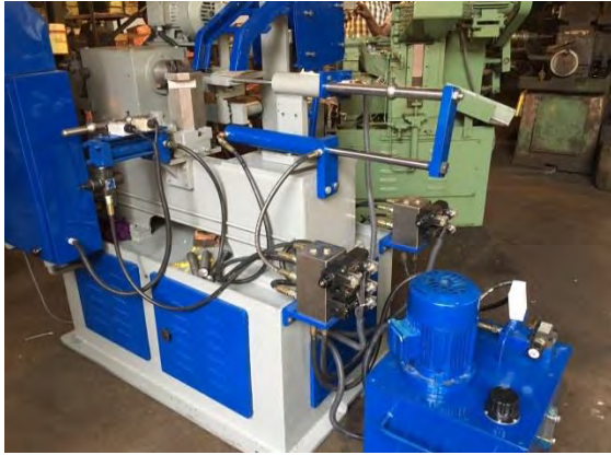
Caption: Special Purpose Machine for Turning Operations at Bharat International
