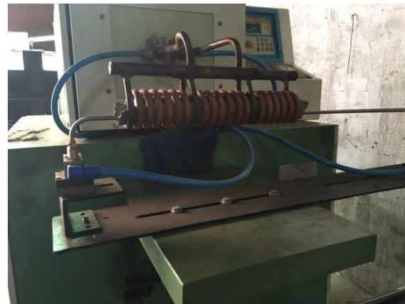
Figure 2.4: Induction heater of capacity 50kW installed at Bharat International
