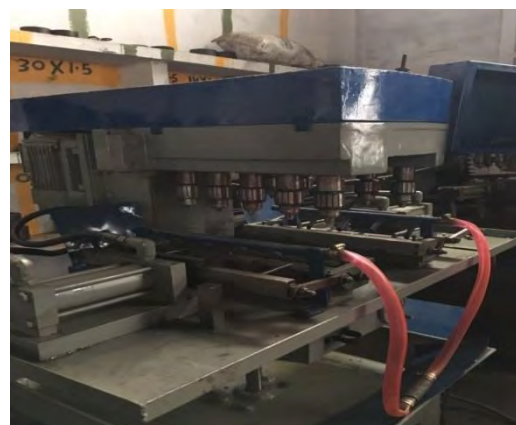
Figure 2.12: Special Purpose Machine (drilling) installed at Bharat International
