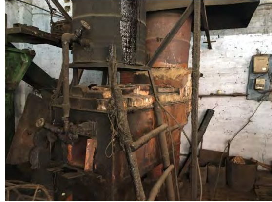
Caption: Conventional Re-heating furnace at Bharat International (Dismantled presently)
