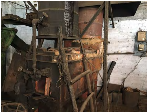
Figure 2.3: Snap shot of FO based re-heating furnace at Bharat International (presently dismantled)
