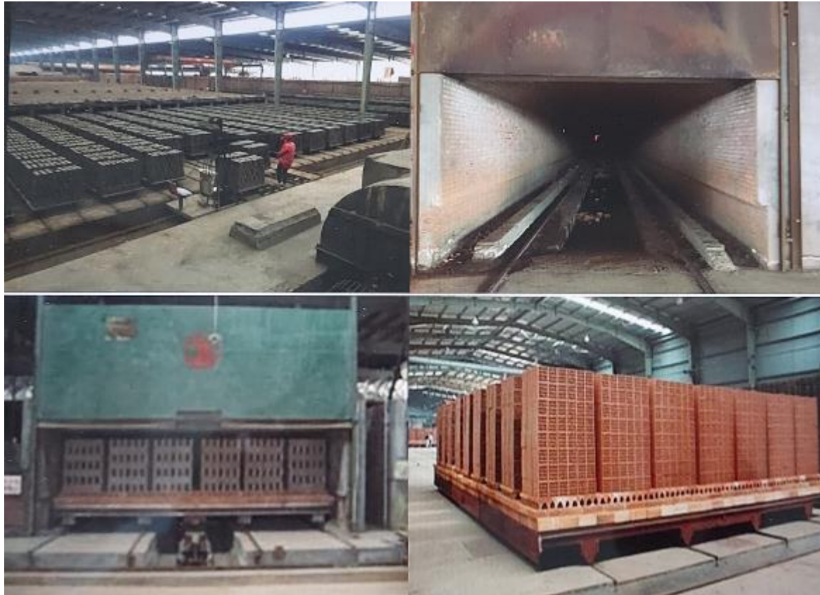
Figure 19 A Tunnel Kiln and Dryer (China)
