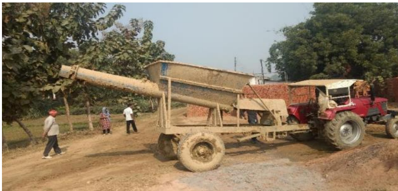
Fig-Pugging of soil using machine
