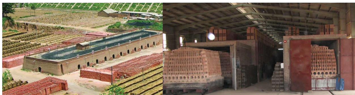
Figure 10 Hybrid Hoffmann Kiln (China) & Tunnel Kiln (Vietnam)
