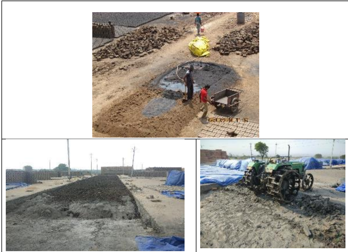
Figure 11 Mixing of internal fuel and fly ash with clay (Maharashtra & Telangana)
