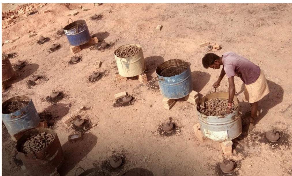
Figure : Use of biomass briquette in a brick kiln
