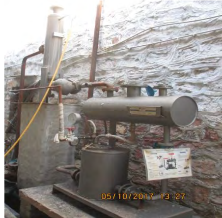
Snap shot of Jet dyeing with condensate recovery system at Manoj Dyeing Pvt. Ltd
