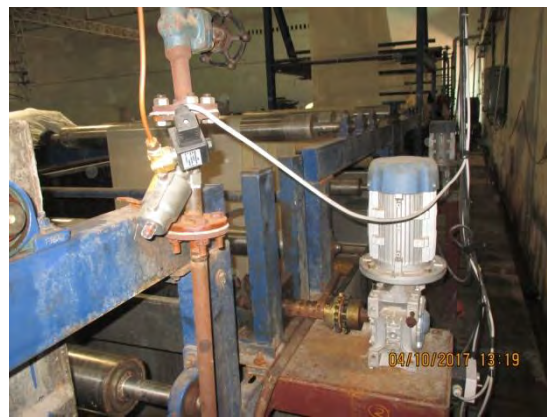
Snap shot of Mercerizing unit which runs with EEf-1 motors with VFD at Shree Rajaram Prints (P) Ltd
