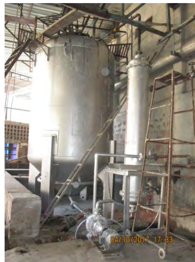
Snap shot of kier boiling unit with waste heat recovery system at Simandhar Fabtex (P) Ltd
