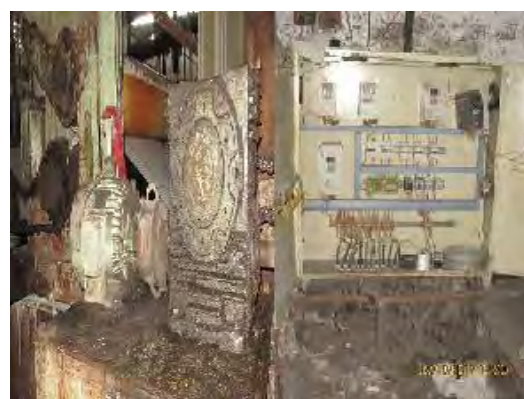
Snap shot of Mercerizing unit which runs with EEf-1 motors with VFD
