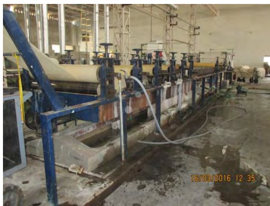
Snap shot of Mercerizing unit running with DC motor at Shree Rajaram Prints (P) Ltd
