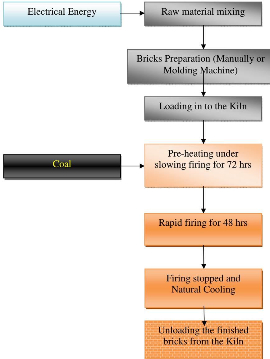
The Refractory Bricks manufacturing process consists of following process involved to complete the one batch production.
