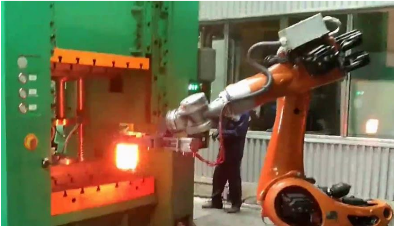
Figure 41 Fully automated forging process
