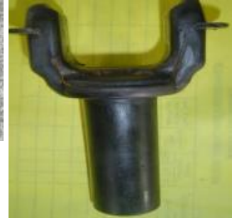
Figure 37 Flashless forging sleeve yoke
