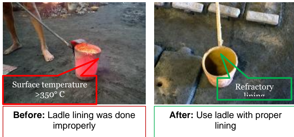
Figure 63 Proper lining of ladle
