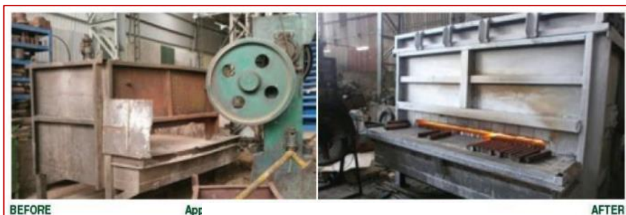
Figure 36: Application of thermo ceramic insulation paint on hot surface
