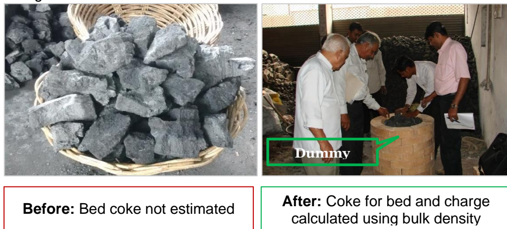
Figure 65 Coke Measurement using Bulk Density
