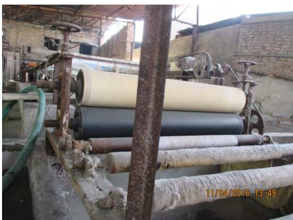
Caustic processing unit at G.G.F. Industries
