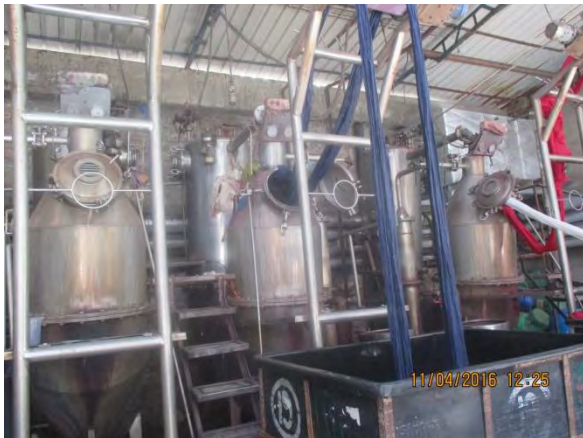
Jet Dyeing Machines at G.G.F. Industries
