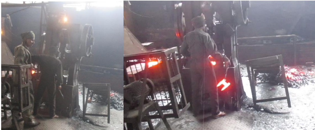
Figure 1.7: Trimming press and material after trimming operation
