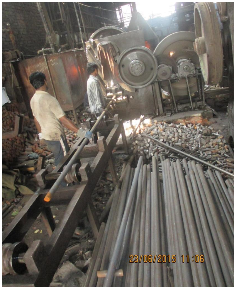
Figure 1.3: Long rods being cut into small pieces using shearing machines
