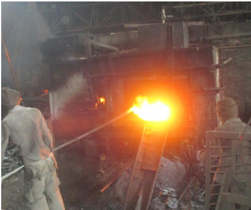
Figure 1.5: Heating of the material inside the oil fired reheating furnace
