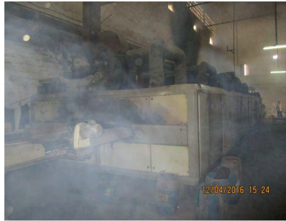
Caption: Finishing operation using Stenter
