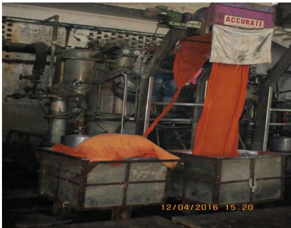
Caption: Polyester dyeing using Jet dyeing machine
