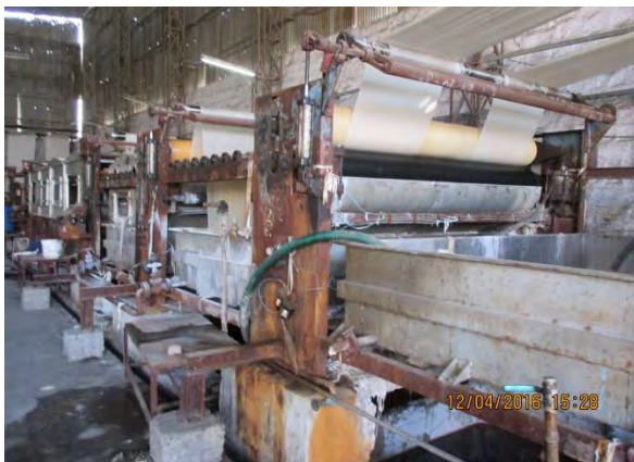
Caption: Caustic processing unit at KB Dyeing
