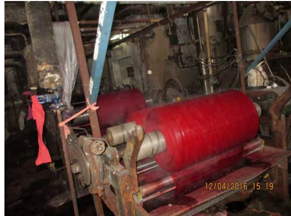
Caption: Cotton fabric dyeing using Jigger Machines
