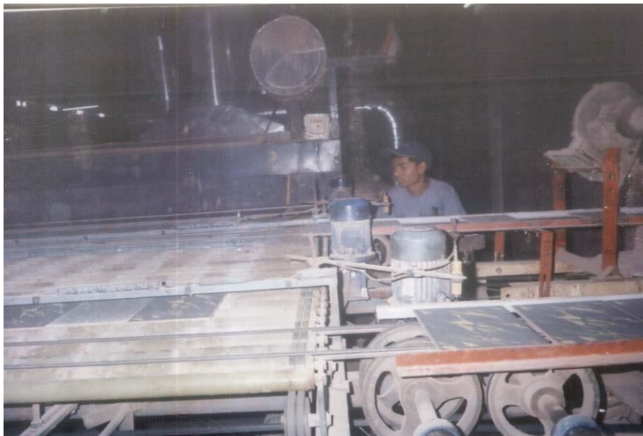
After Glazing & Printing again heat in Kiln machine
