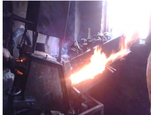
Figure 2.1: Oil fired re-heating furnace (Presently dismantled)
