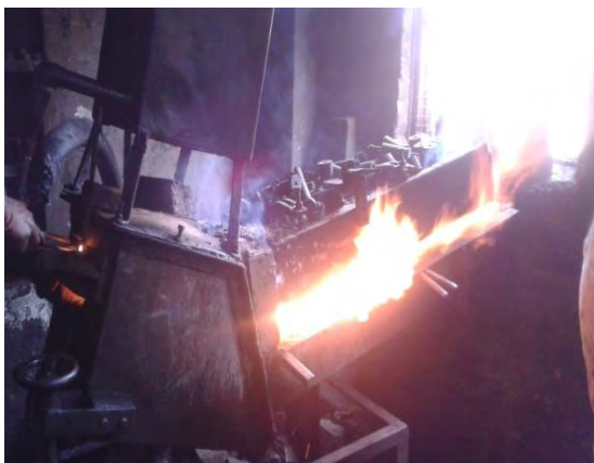
Figure 2.4: Snap shot of FO based re-heating furnace at NN Products (India) (presently dismantled)
