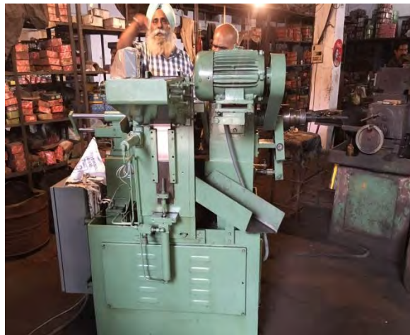
Figure 2.11: Special Purpose Machine (Long Hydraulic Thread) installed at NN Products (India)
