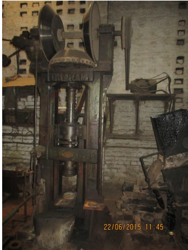
Forging press being used in the unit
