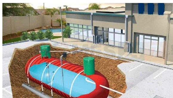
Figure 91: Freshwater saving by rainwater harvesting
