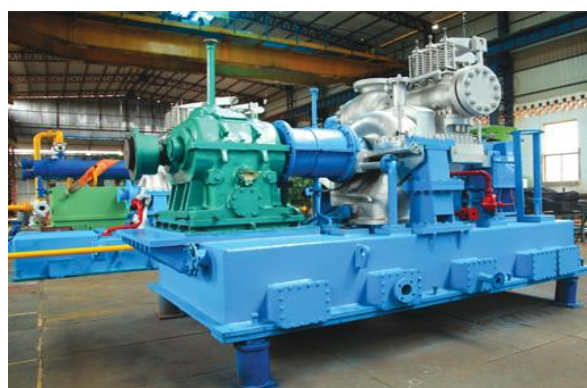
Figure 106 Back pressure turbine
