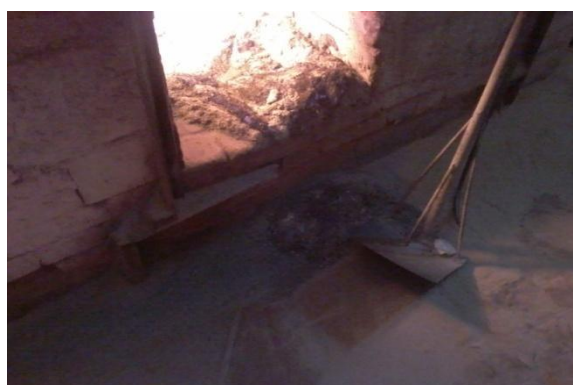
Figure 15: Ash removal opening in roaster
