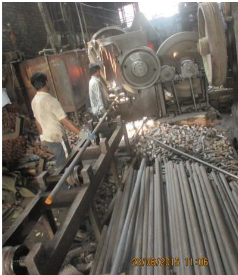
Figure 1.3: Long rods being cut into small pieces using shearing machines
