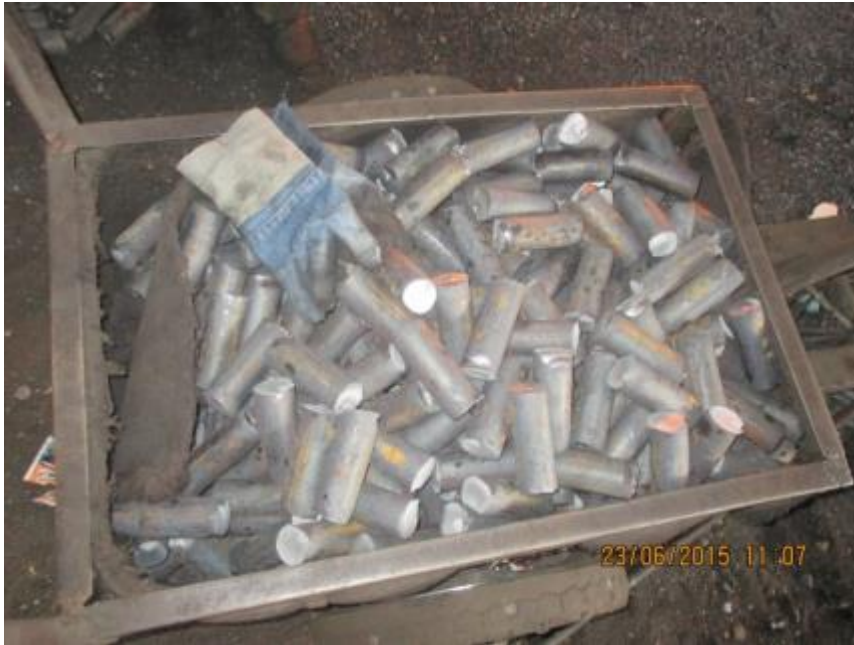
Figure 1.4: Cut pieces being put into the furnace
