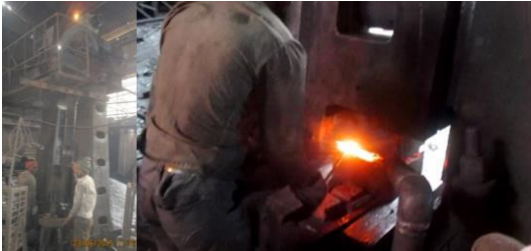
Figure 1.6: Forging press and heated material being forged in the press
