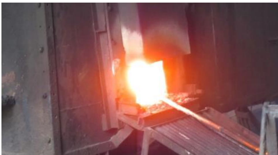
Figure 2.3: Heated material piece being taken out from furnace for forging
