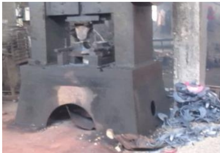
Figure 1.8: Forging press installed in the unit
