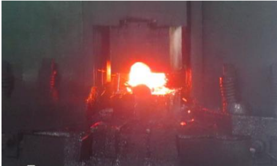
Figure 1.7: Heated material being forged in the forging press
