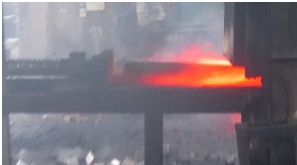
Figure 1.5: Cut pieces being put into the furnace
