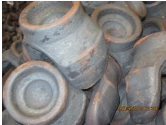
Figure 1.11: Material piece before shot blast operation
