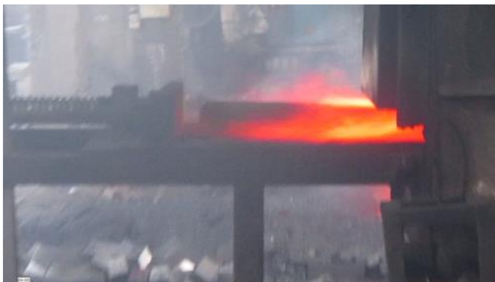
Figure 2.2: Cut pieces being put into the furnace
