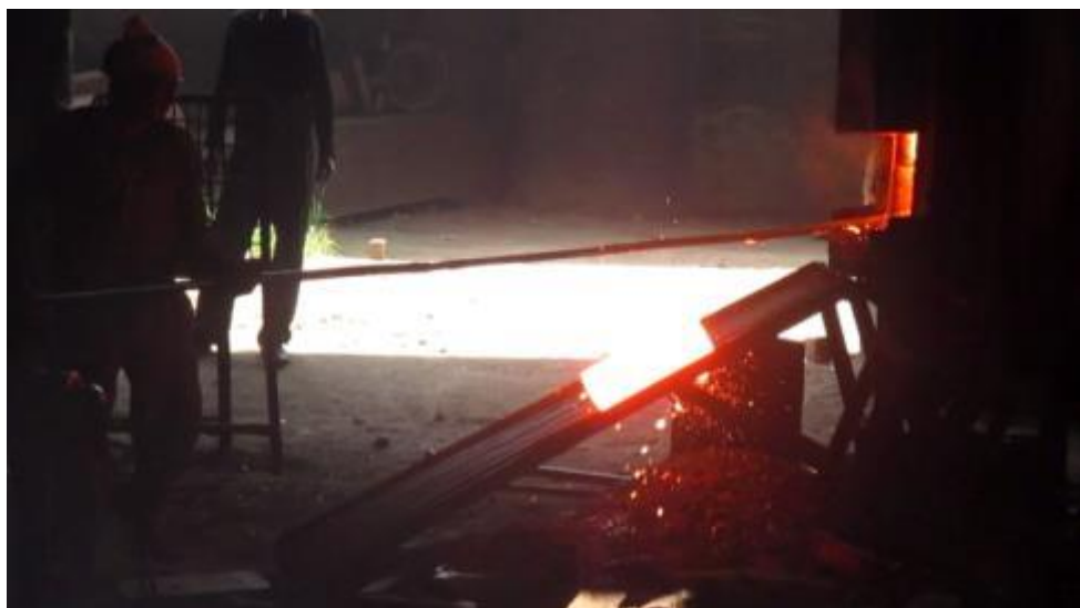
Figure 1.6: Heated material taken out of the furnace
