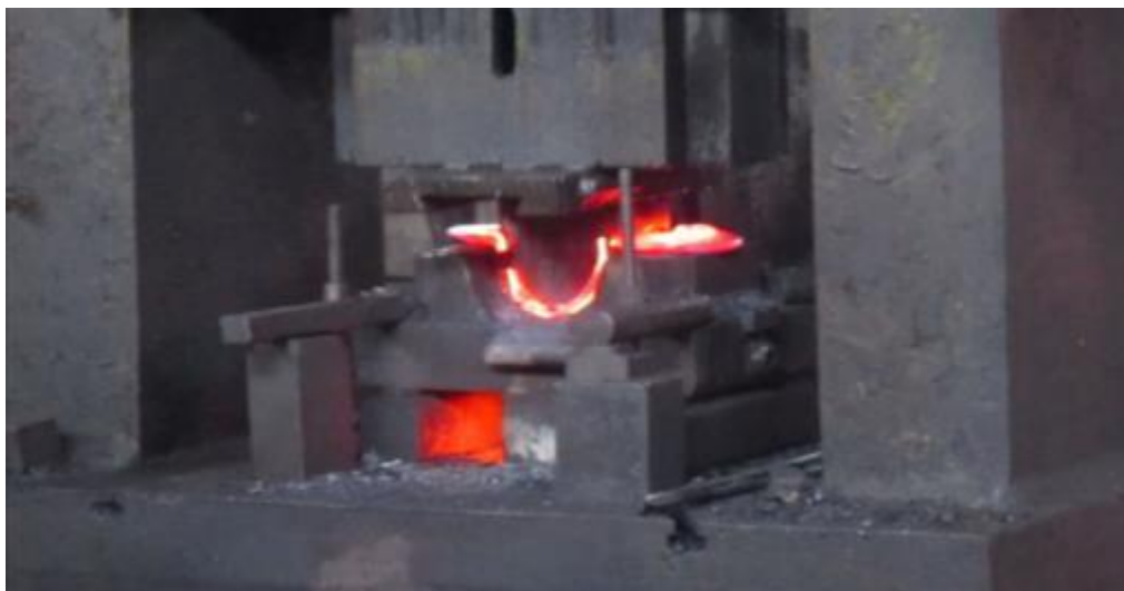
Figure 1.9: Material being processed in the forging press
