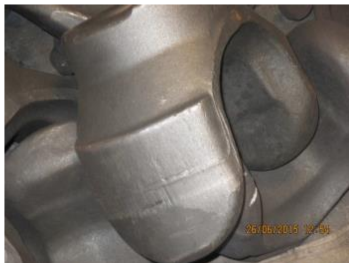
Figure 1.12: Material piece after shot blast operation
