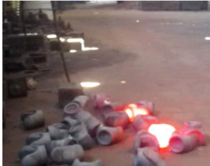
Figure 1.10: Heated material after operation in forging press lying for natural cooling
