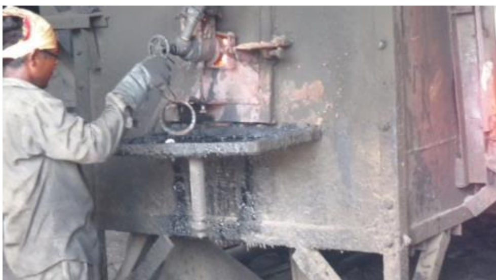
Figure 2.4: Manual control of fuel in the furnace
