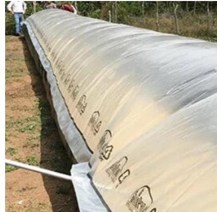
Figure 70: Tunnel based solar paddy dryer
