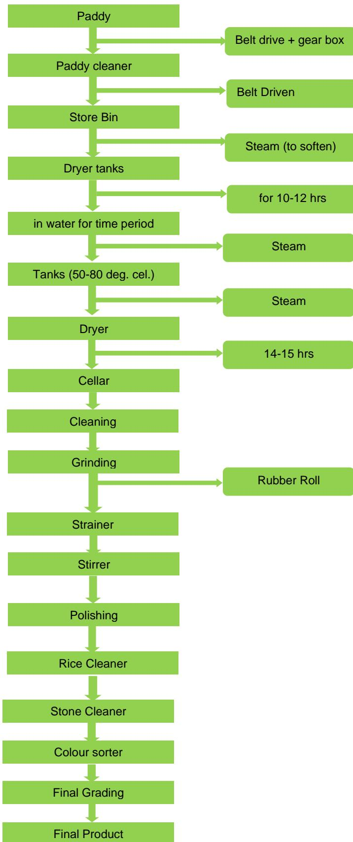
Figure 36: Process flow diagram of typical rice mill unit
