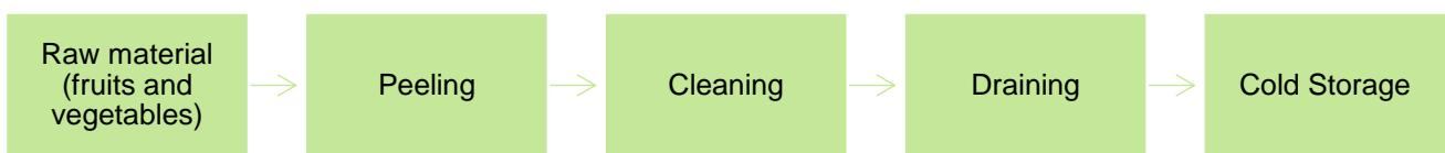
*Figure 40: Process flow diagram of Frozen Fruits and Vegetables*
