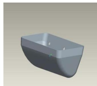
Figure 43: Iron and Plastic bucket for elevators
