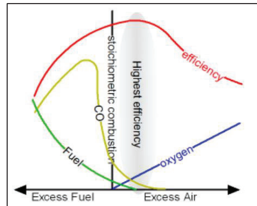
Figure 73: Efficiency of the boiler vs fuel and air supplied
