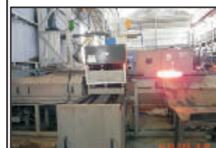
Induction end bar heater in operation
