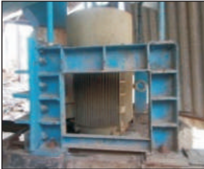
Energy Efficient Vertical Pulper Motor 150 HP
