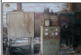
Fuel oil fired end bar reheating furnace
