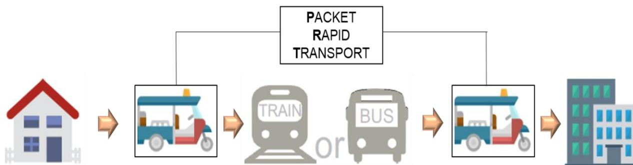
The PRT system consists of electric three wheelers that can be hailed through a mobile app during off-peak hours, and during rush hours they operate in a specific neighbourhood around metro, bus or suburban train stations.
