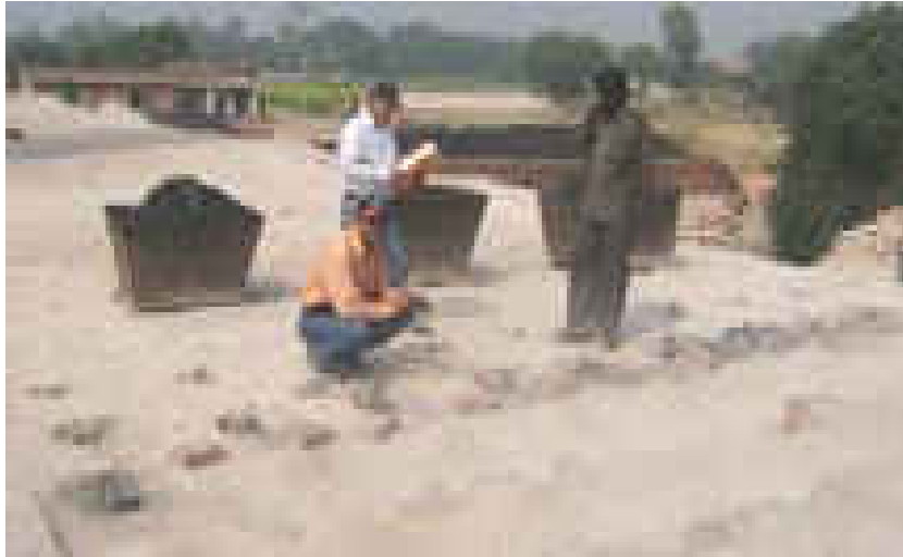
Image 5: Combustion Zone with lines covered by metallic lids
