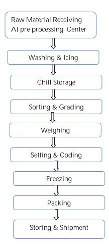
From the flowchart, it can be inferred that the energy intensive steps in the process are the freezing and the storage. Freezing alone accounts for nearly 75% of all the electricity consumed in the unit.
