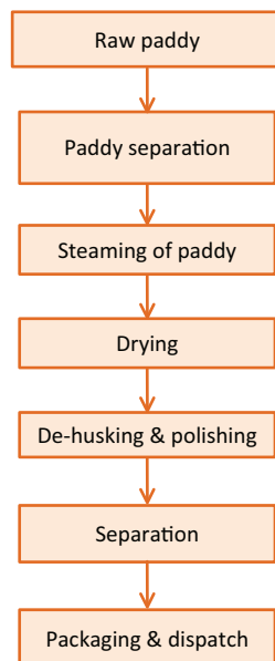
Figure 6.28: Production process of parboiled rice
